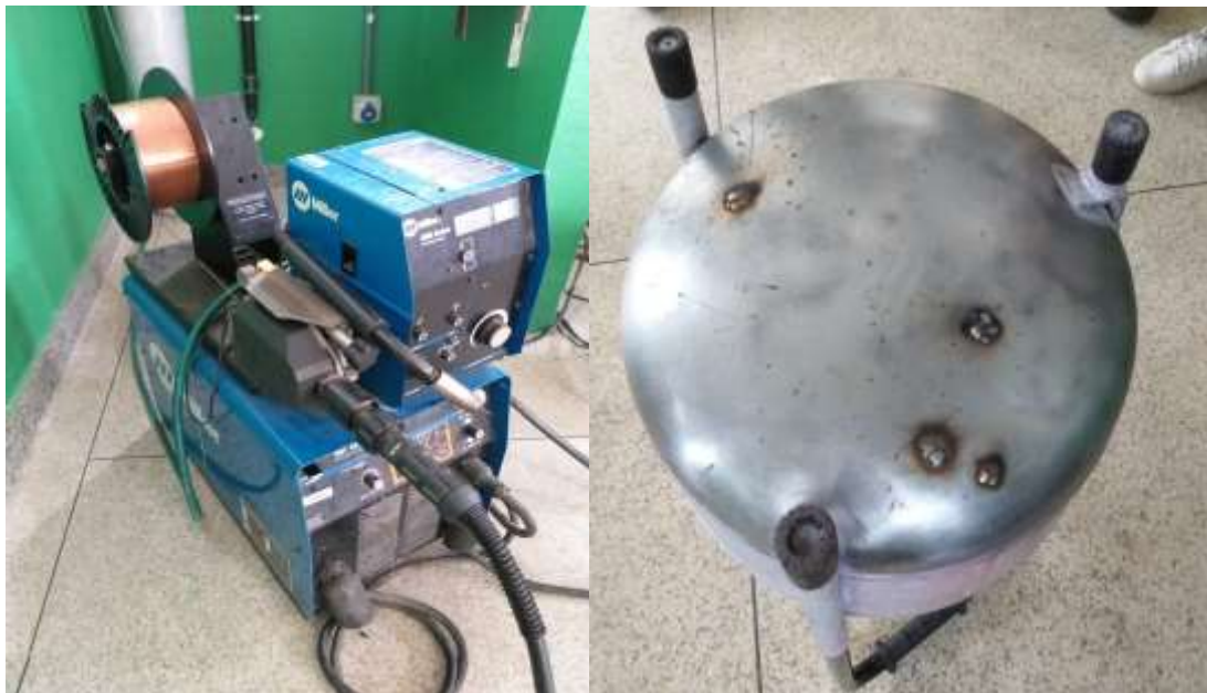
Figure 9 - MAG welding equipment and reservoir after welding
