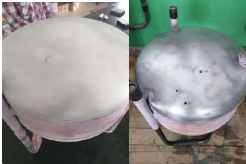
Figure 8 - Reservoir bottom after developer application and drilling
