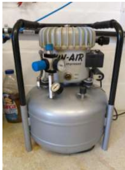
Figure 11 - Reservoir after cleaning and painting
